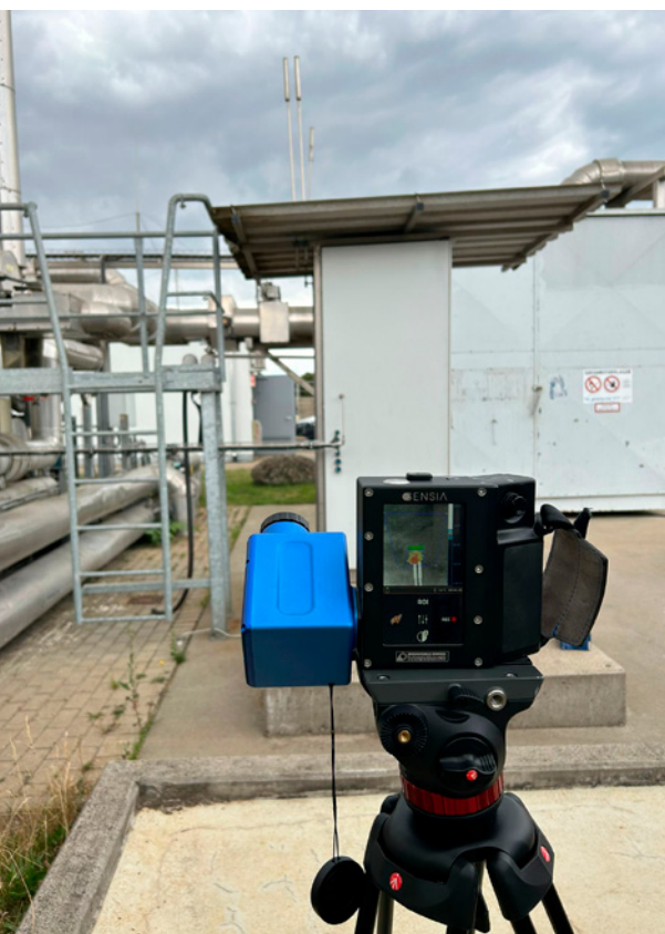
Fig. 23: Detection and quantification of methane emissions using a q-OGI gas imaging camera at a pressure relief device
