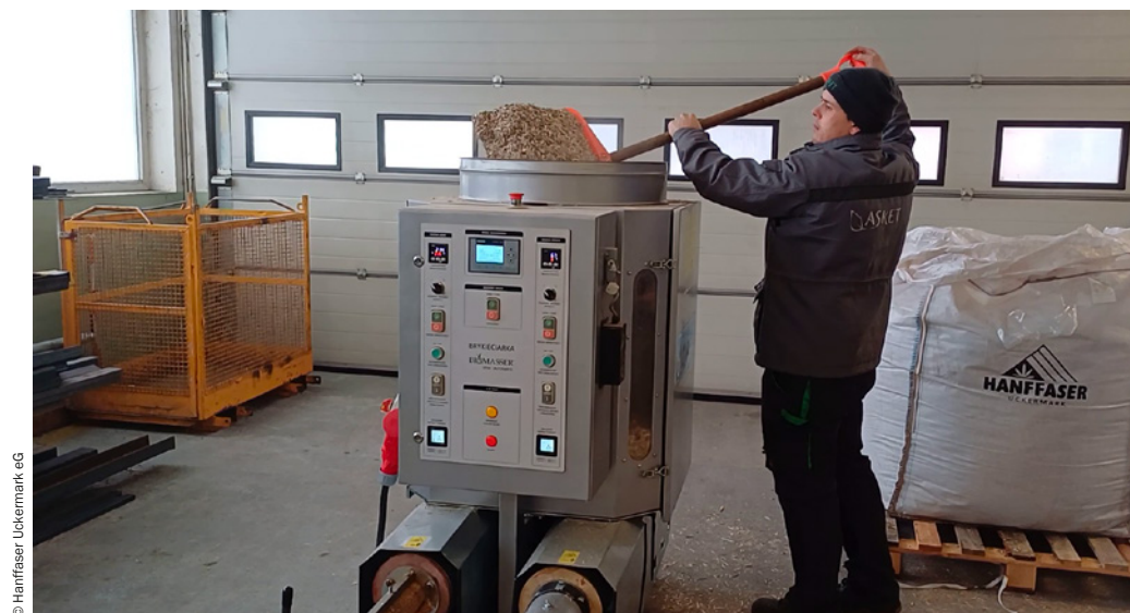
Fig. 53: Pressing hemp briquettes using a thermal process
