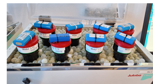
Figure 2: Anaerobic digestion tests with process water from HTC of sewage sludge
