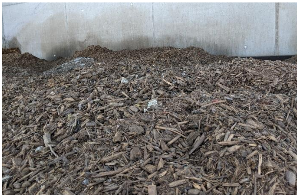
The feedstock for biochar includes small plastic pieces that will be completely combusted during pyrolysis.
