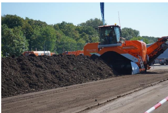
High-tech compost turner Backhus by Eggersmann: It is partly automated (GPS), has a climatized operator's cabin including a fridge etc... It can switch between side and back release of the compost. Windrow width 5 m
