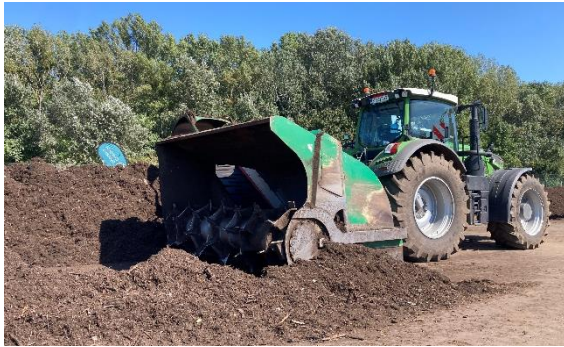
Compost turner towed by a tractor. The compost is released to the side.
