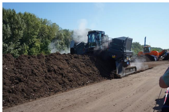
Partly automated compost turner by KompTech. It has similar features as the Backhus.
