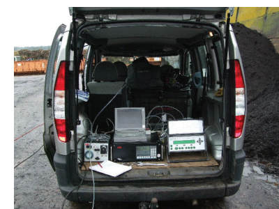
Exhaust air measuring technology with sampling pump and analysers as well as online acquisition of measured values
