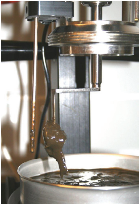
Figure 37: Adherence of solids to the surface of the ball (Source: BREHMER)
