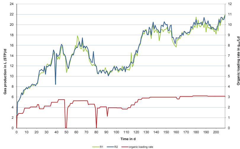
Figure 79: Gas production and organic loading rate of two continuous fermentation tests in parallel test (Source: DBFZ)
