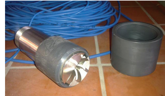
Figure 49: Sensor head of the vane anemometer for the measurement of the velocity in industrial scale biogas plants; built by Fraunhofer UMSICHT (Source: TU Berlin)
