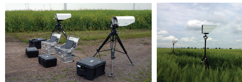
Figure 21b: To the left: laser spectrometer, to the right: reflector modules (Source: DBFZ)
