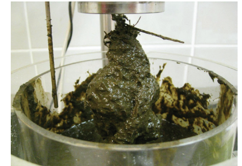
Figure 35: Wrapping of the vane shaft with long fibre substrate components (Source: BREHMER)
