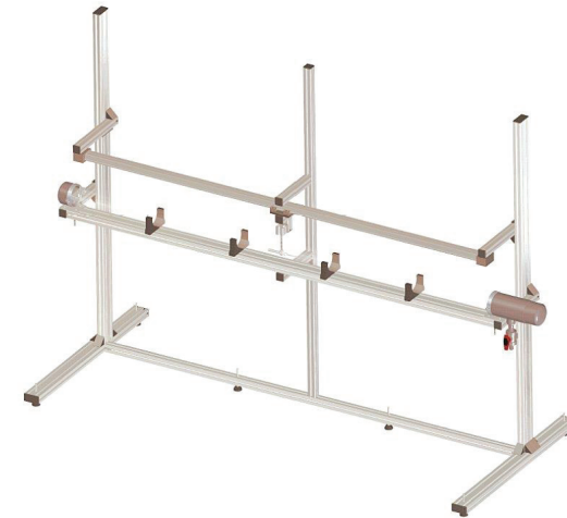
Figure 54: Towing-channel for the calibration and determination of the constants of a film sensor
