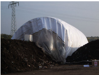
Exhaust air from the wind tunnel with the sampling hose (rear view of the wind tunnel)
