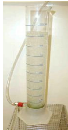
Figure 6.3-2: Foam generator with model foam (Source: UFZ)
