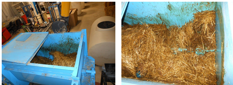
Figure 8.7-5: Paddle mixer used to prepare substrate mixtures for dry digestion (Source: InnoTech)
