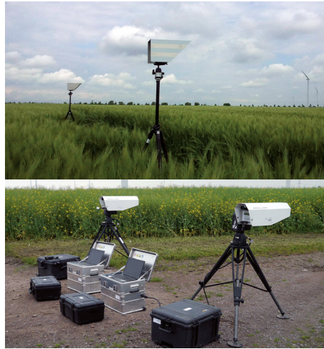
Figure 5.6-1b: To the left: reflector modules, to the right: laser spectrometer (Source: DBFZ)
