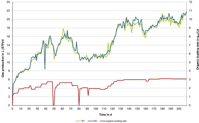
Figure 7.4-4: Gas production and organic loading rate of two continuous fermentation tests in parallel test (Source: DBFZ)
