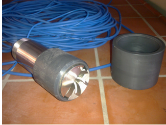
Figure 6.6-1: Sensor head of the vane anemometer for the measurement of the velocity in industrial scale biogas plants; built by Fraunhofer UMSICHT (Source: TU Berlin)
