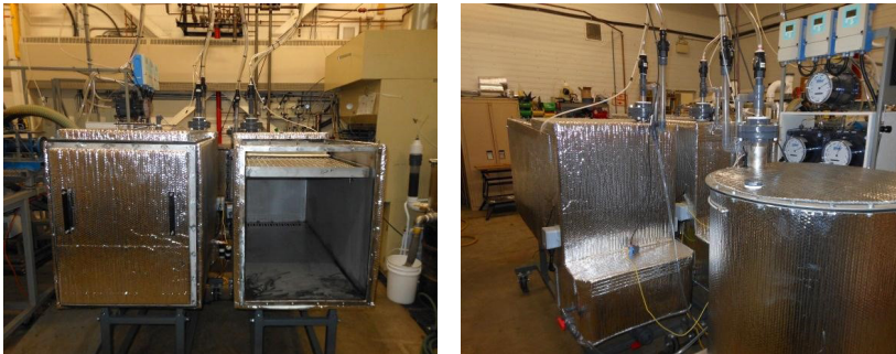
Figure 8.7-1: Dry batch digestion pilot plant at AITF. The pictures show the front of the system (left) and back (right) with a round percolation digester in the back (Source: InnoTech)
