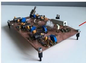
Heater control electronics with digital potentiometer
