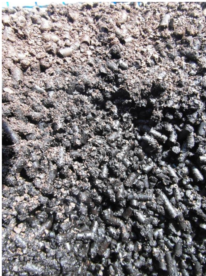
Figure 17: Cross section of top of flat pile, showing high fines layer above wetter pellet
