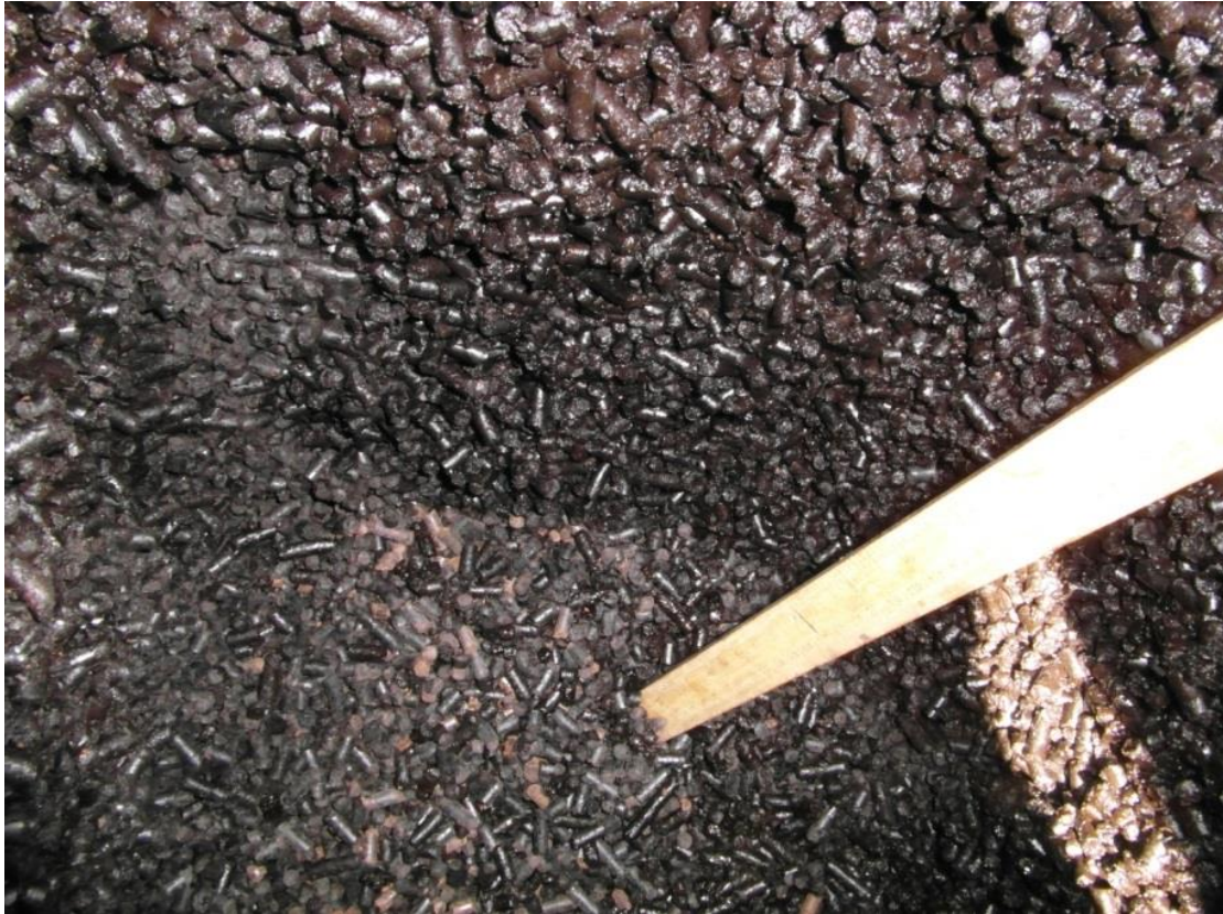
Figure 13: Sampling "pit" in flat pile
