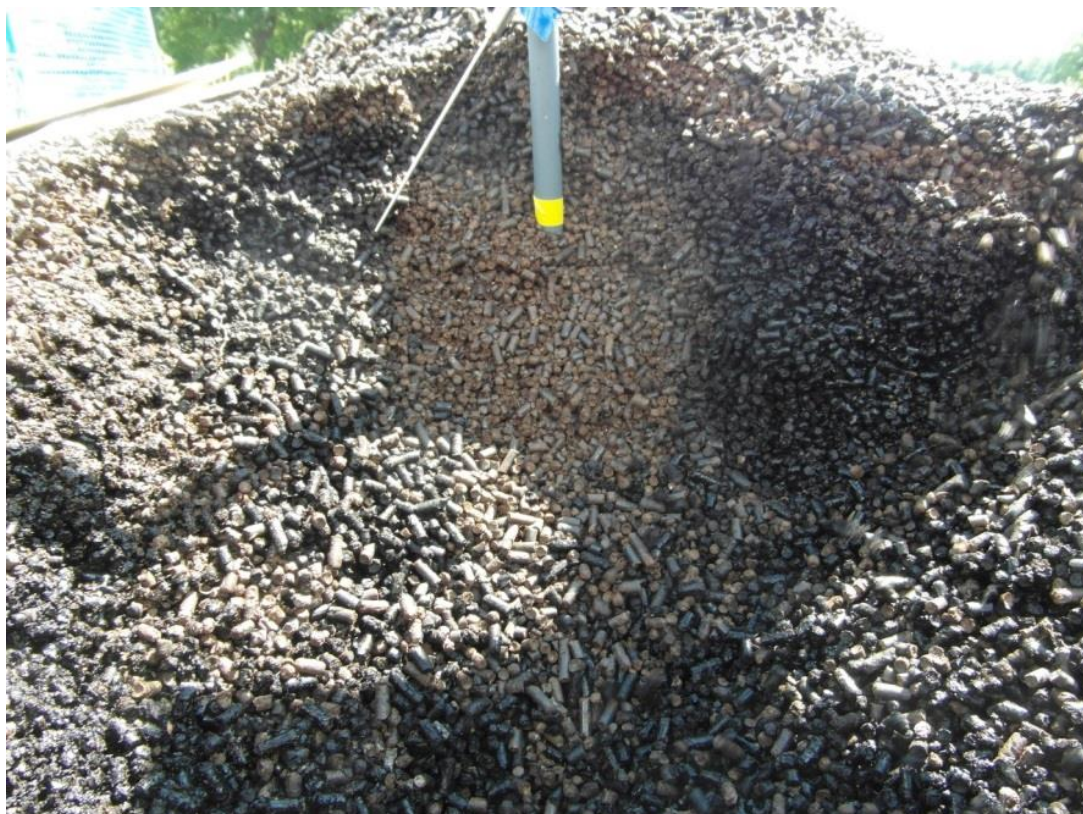
Figure 19: Interior of peak pile during dismantling
