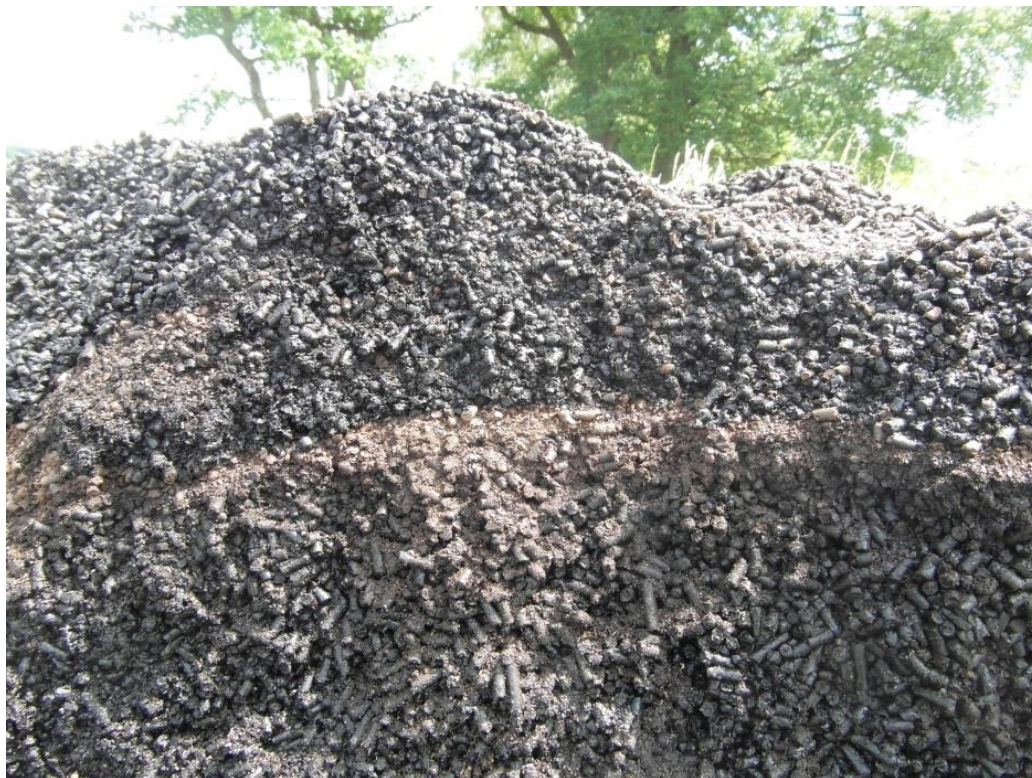
Figure 18: Vertical face of flat pile during dismantling, showing areas of pellets with different moisture contents
