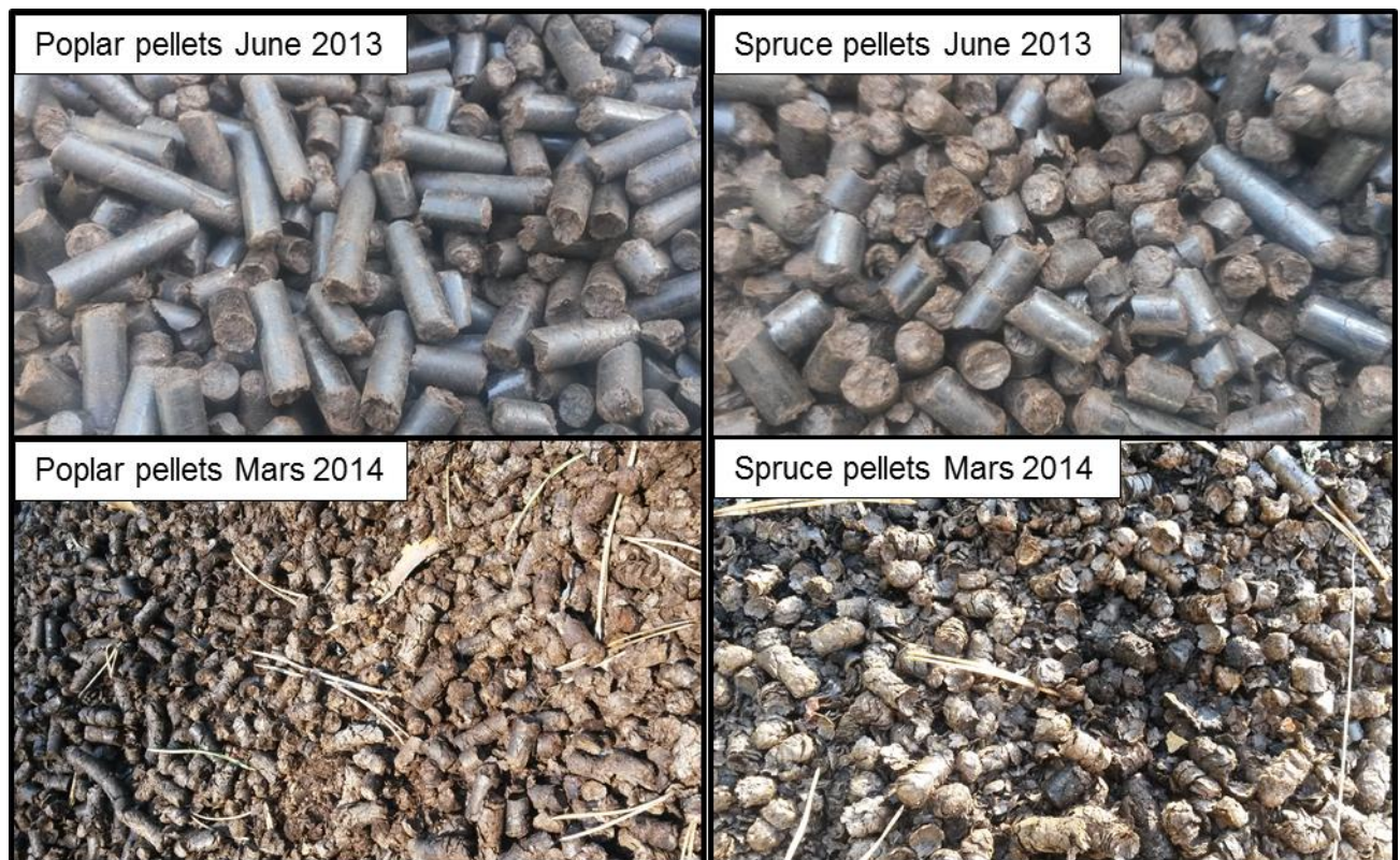
Figure 43: The poplar and spruce pellets at start and end of the 9 month outdoor storage period. The pellets close to the surface have a considerably rougher appearance compared to the original conditions. There is also a significant amount of fines from disintegrated pellets close to the surface.
