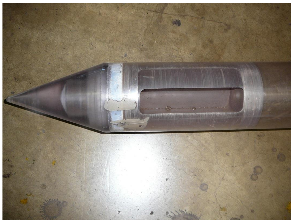
Figure 8: Spike of sampling spear, showing rotating trapdoor (half open)
