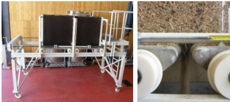
Bridging properties: Movable floor with expandable opening (direct measurement)
