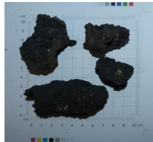
Ash agglomerates (underfeed boiler)
