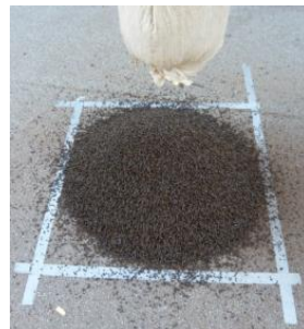
Bridging properties: Movable floor with expandable opening (direct measurement)
