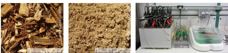
Fig. 2: Poplar wood chips and fibres obtained after extrusion and BMP testing device AMPTS II
