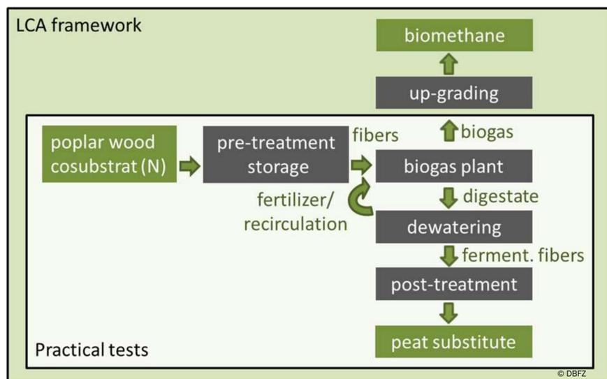
Fig. 1: Schematic draft of the process concept
