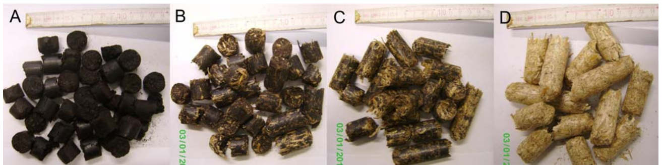
Abbildung 5: Hergestellte Biomassepellets (A: 100% Traubentrester; B: 30% Traubentrester / 70% Miscanthus; C: 70% Traubentrester / 30% Miscanthus; D: 100% Miscanthus)
