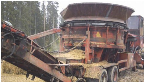
The mobile pelletizing process: The complete bale can be put to hammer mill. The press is a ring die of CPM.
