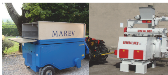
Picture 1: grapevine pruning harvester (left) and pelletizing mobile machinery (right).
