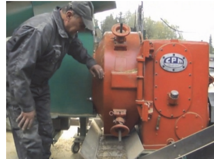
The mobile pelletizing process: The complete bale can be put to hammer mill. The press is a ring die of CPM.
