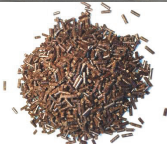
Figure 1: Grape marc residues (above) and pellets made of 70% grape marc / 30% vine pruning pellets (bottom)
