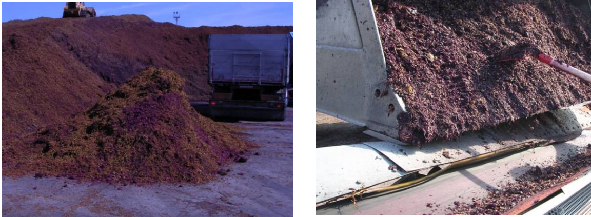
Figure 22: Grapevine residues heap (left) and conveyor belt for movement of the material (right) Source: Giuseppe Toscano, Italian Thermotechnical Committee (CTI)
