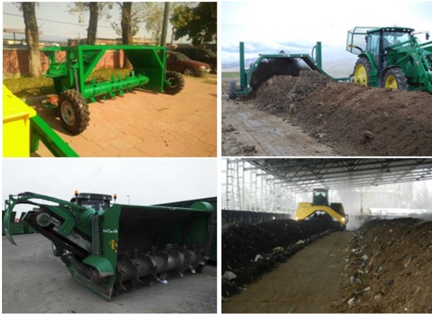
Figure 19: Examples of turner devices of varying size and capacity used for open windrow composting (Picture sources: INTECUS)
