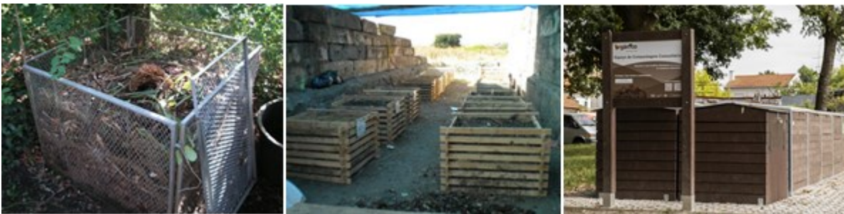
Figure 17: Examples of simple composting units for individual home composting and set up as a village-composting facility (Picture sources: INTECUS / LIPOR/Community of Porto, 2021)
