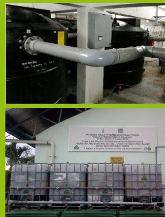
c) Fermentation tanks get filled with processed food waste to which market grey water and the inoculant (bokashi) are added
